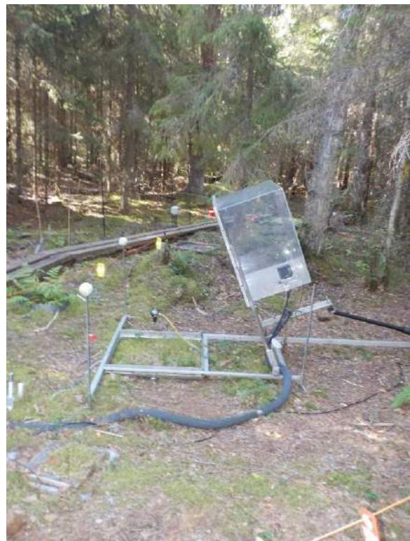
Figure 12. Left: ditch recently deepened in a commercially successful drained peatland at Lattosuo. Right: automatic chambers sampling CO 2 emissions within the forest to supplement measurements being carried out using eddy covariance
