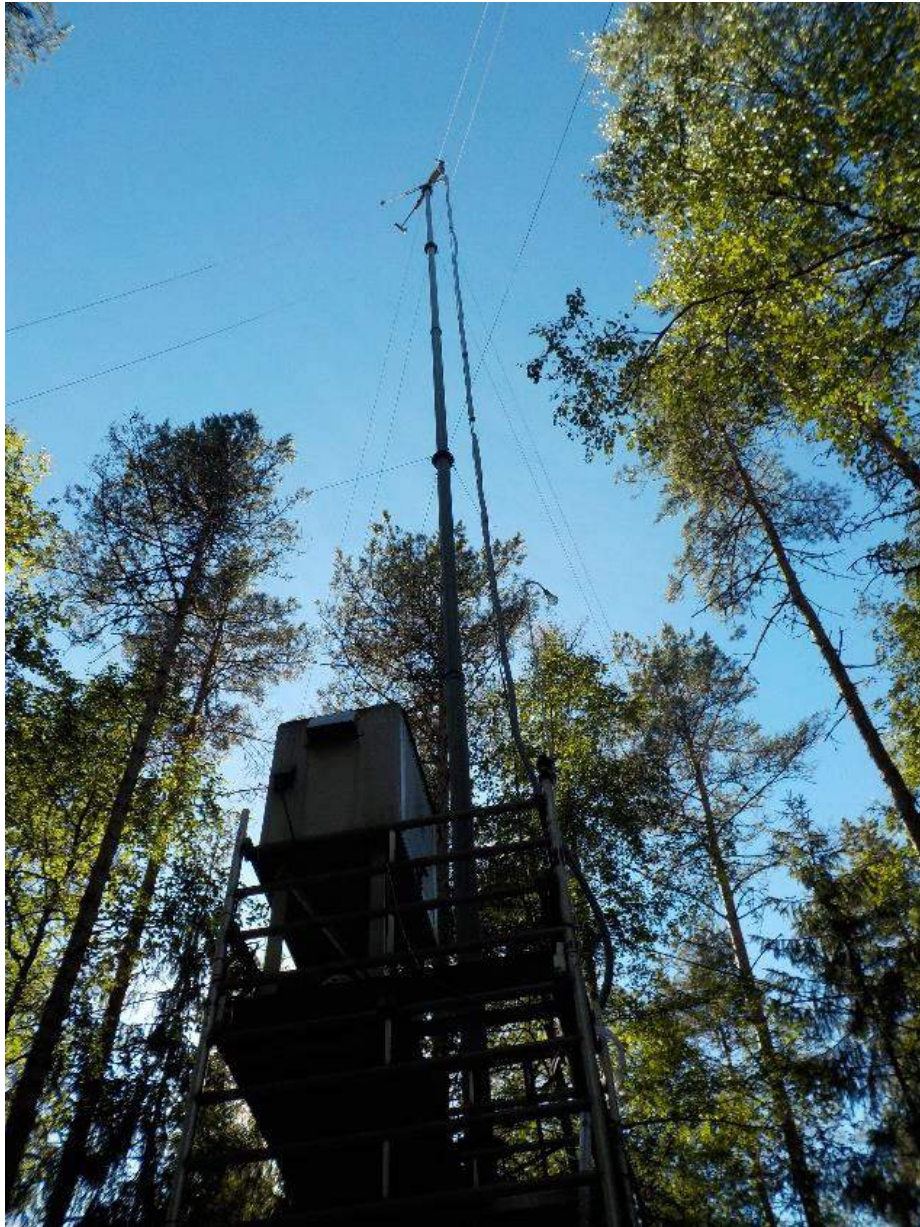
Figure 13. Eddy covariance tower at Lettosuo monitoring ecosystem CO 2 balance in real-time - eddy covariance towers in forested peatlands are much taller in order to capture the CO 2 flux from the tree canopy
