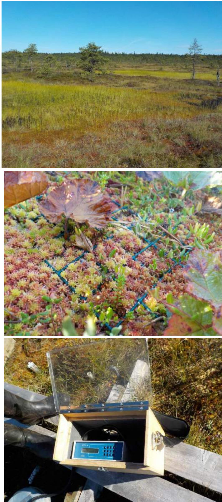
Figure 6. Top: pristine peatland at Torronsuo. Middle: nets used to measure the growth of Sphagnum , a good indicator for wetland restoration. Bottom: Environmental Gas Monitor used to take CO 2 measurements from the site in real time -it is not possible to measure CH 4 in situ therefore gas samples have to be taken back to the lab
