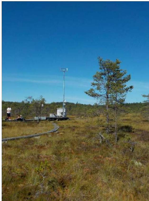
Figure 10. Eddy covariance tower at Tervalamminsuo which is able to measure real-time whole ecosystem CO 2 flux
