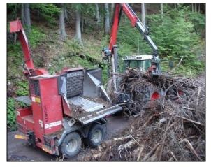
Picture 13 PTO driven wood chipper
