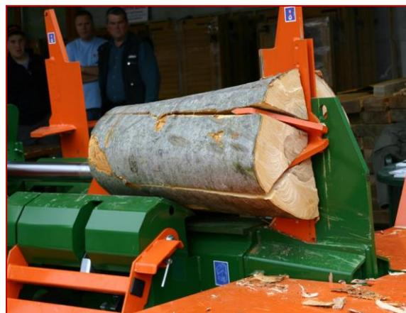
Picture 10 Hydraulic horizontal splitter
