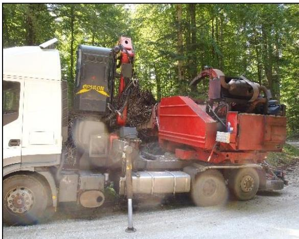
Picture 16 Wood chipper on the truck
