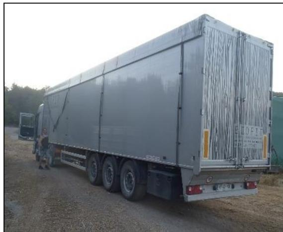
Picture 17 Truck with cargo floor trailer
