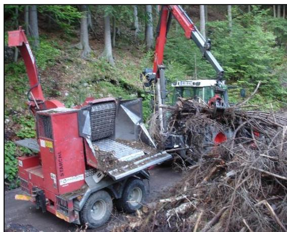
Picture 13 PTO driven wood chipper
