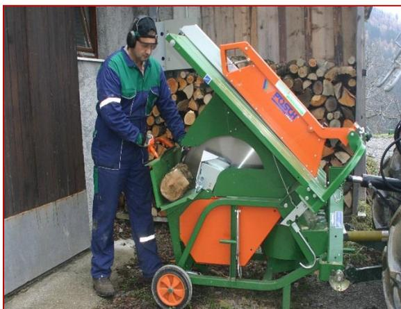
Picture 9 Tractor driven circular saw
